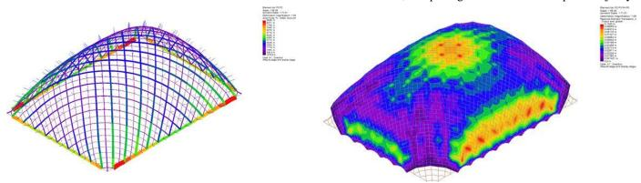
Fig. 8. Forces in the steel cable framework
