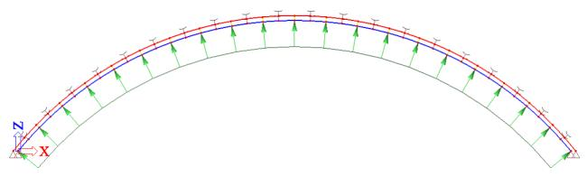
Figure 5: Two-dimensional FEM model to study the interaction the hybrid structure, with the blue cable representing the air-supported dome and the red cable representing the shade
