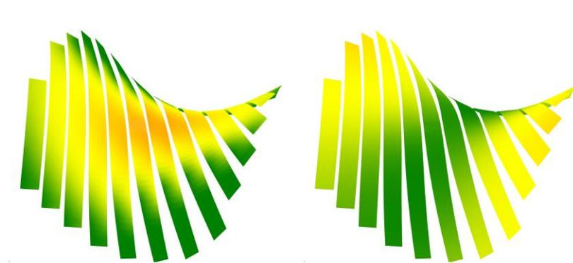
Figure 9. Left: Graphical display of the amount of bending; green indicates a large bending radius. Right: Graphical display of surface deviation at the center curve of the strips; green indicates a small deviation between the original surfaces and the triangulated strips.
