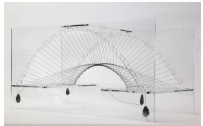
Figure 4: Final wire model of the cable net
