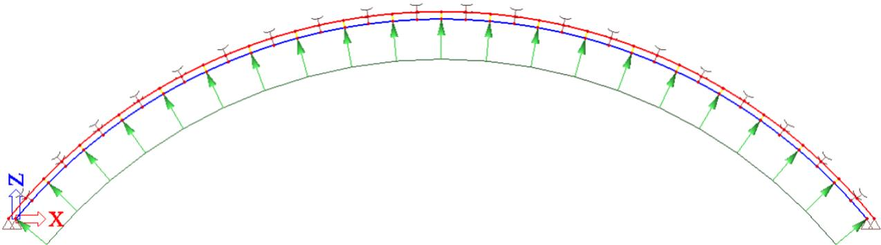
Figure 5: Two-dimensional FEM model to study the interaction the hybrid structure, with the blue cable representing the air-supported dome and the red cable representing the shade
