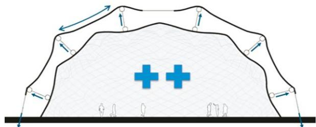
Figure 3. Section of the Shade Dome, showing the overpressure in the air-supported dome (blue plusses) and the forces (blue arrows) being transferred via the spacers to the shade.
