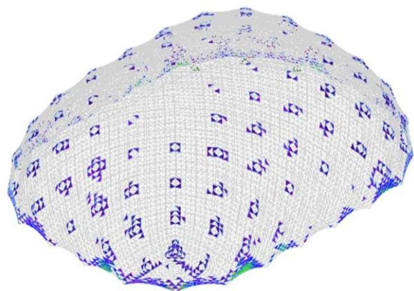
Figure 6: Three-dimensional FEM model of the prototype, with the coloured elements indicating a difference in principle stresses of more than a factor 10
