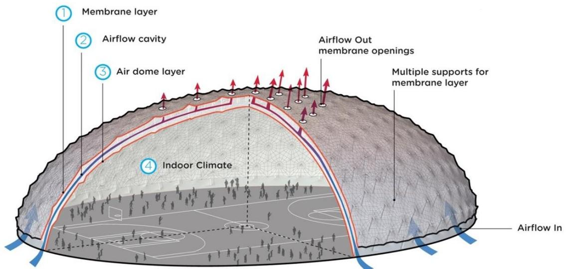
Figure 1. Functional Diagram of the Shaded Dome showing the buffering effect and the airflow in the cavity.
